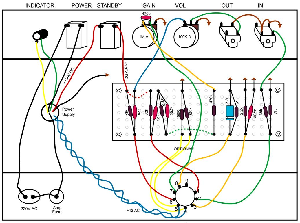
Alternative heater connection suitable for 6.3V supply
